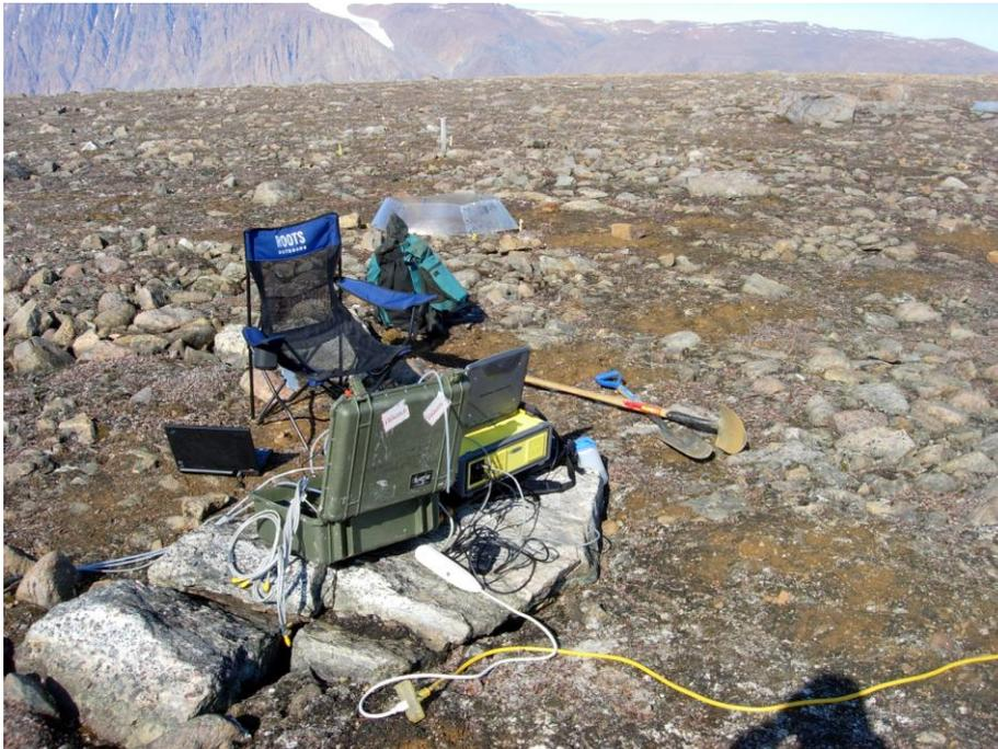
Gaset DX4015 used for greenhouse gas monitoring.
